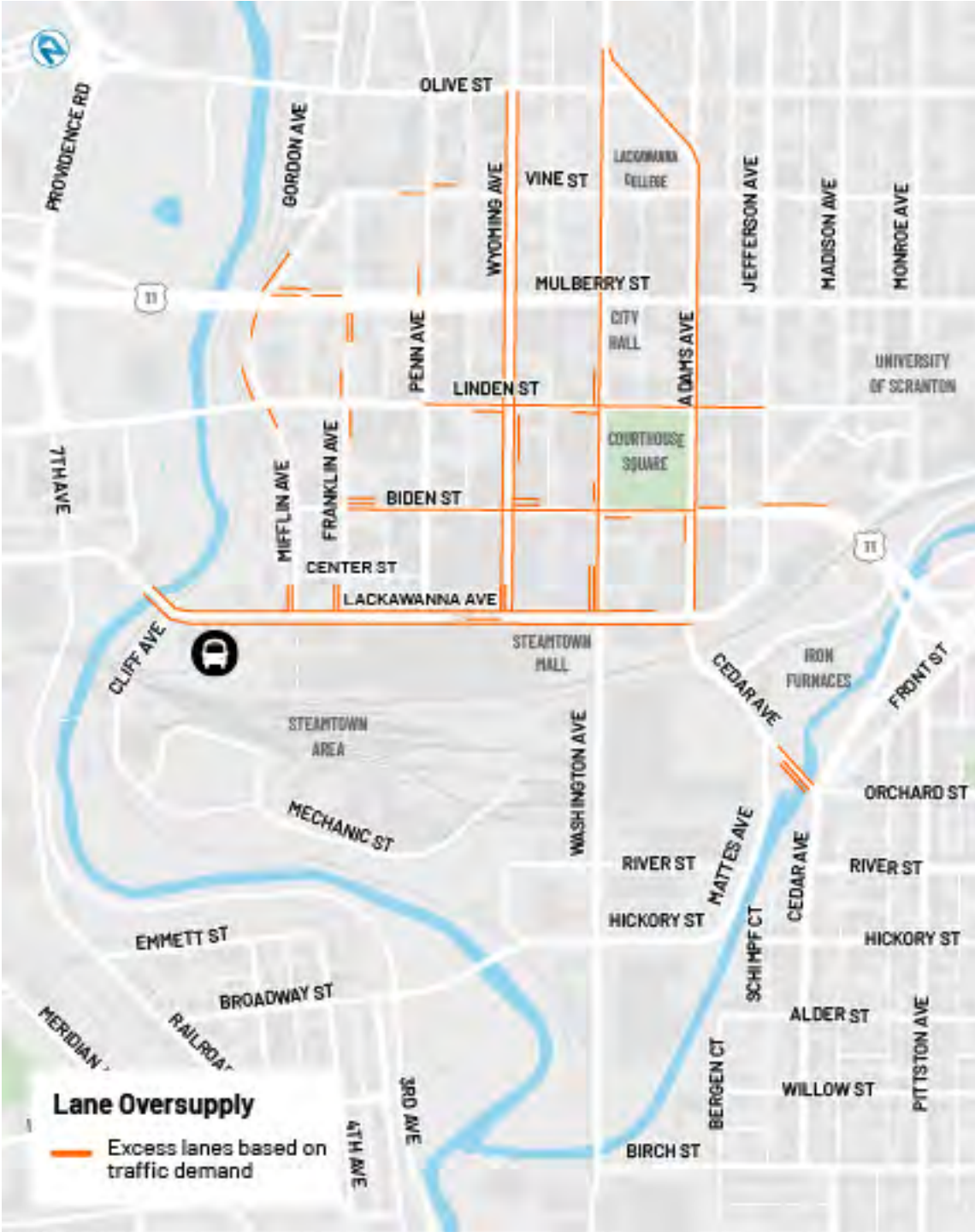
The current oversupply of driving lanes in downtown Scranton.
